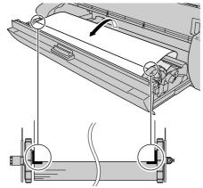
**11** While pressing down on the center of the roll media, turn the roll holder in the direction shown in the illustration below to remove all slack from the media.
